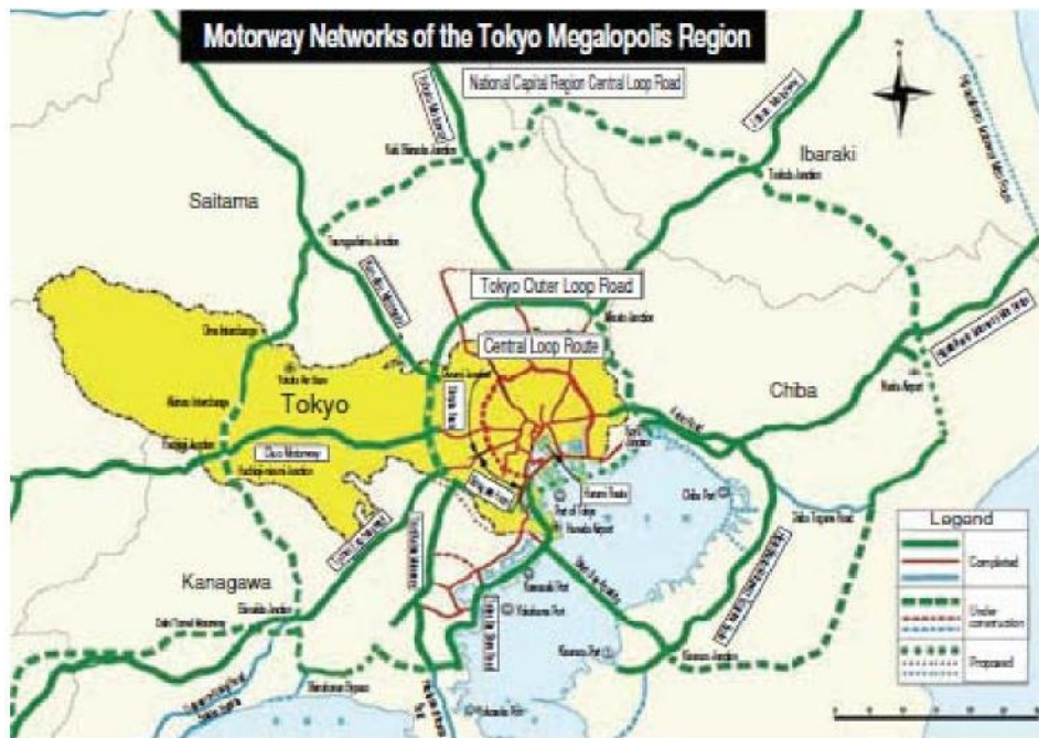
Figure 6: Three circular expressways under construction or planning in the Tokyo megalopolis region
